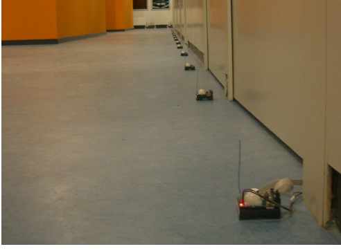
Fig. 2. Placement of 16 ESB Nodes on our Office Floor
