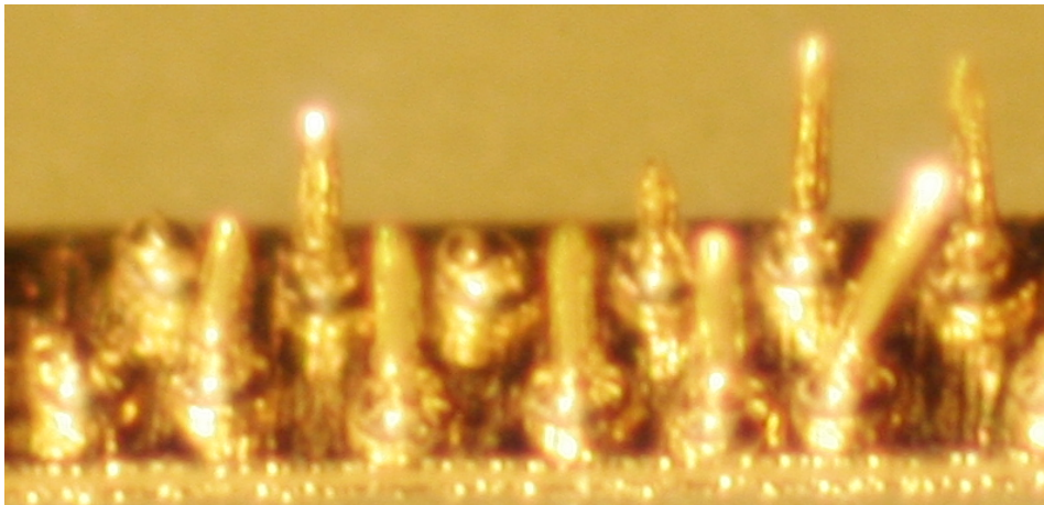
Figure 6.4: Photograph of bumps with long tails caused by non uniform rip-off of the 25\mu m wire.
