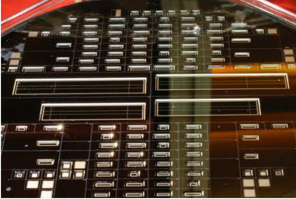
Figure 7.8: Photograph of the back side of the first 50\mu m thin PXD6 wafer. The cavities where the silicon is etched back are clearly visible. [63]
