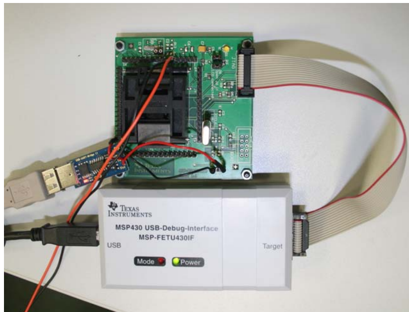
Figure 12.1: MSP430FET development board: supports a standalone ZIF socket target board (64-pin LQFP package) used to program (flash emulation tool (FET)) and debug the MSP430 \mu C in-system through the JTAG interface or the Spy Bi-Wire (2-wire JTAG) protocol.
