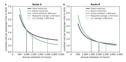
Figure 1: Levelized cost per passenger-mile. **a,b**, This figure shows the levelized cost per passenger-mile of diesel and electric transit buses for (**a**) Route A and (**b**) Route B.
