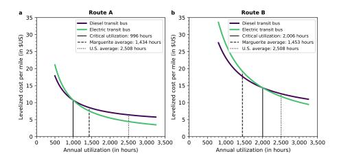
Figure 2: Levelized cost per mile. **a,b**, This figure shows the levelized cost per mile of diesel and electric transit buses for (**a**) Route A and (**b**) Route B.
