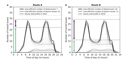
Figure 3: **Cost-efficient vehicle fleets. a,b**, This figure shows the cost-efficient number of diesel and electric transit buses for the hourly load profile of Marguerite in 2019 if hypothetically all routes exhibited a duty cycle of either (**a**) Route A and (**b**) Route B.
