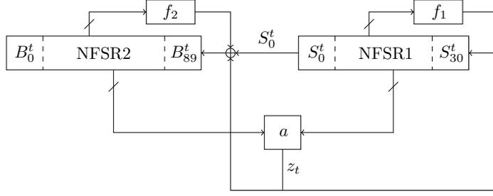
**Figure 2:** LIZARD in phase 2 of the state initialization.
