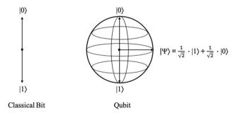
Fig. 1 Illustration of a classical bit and a qubit
