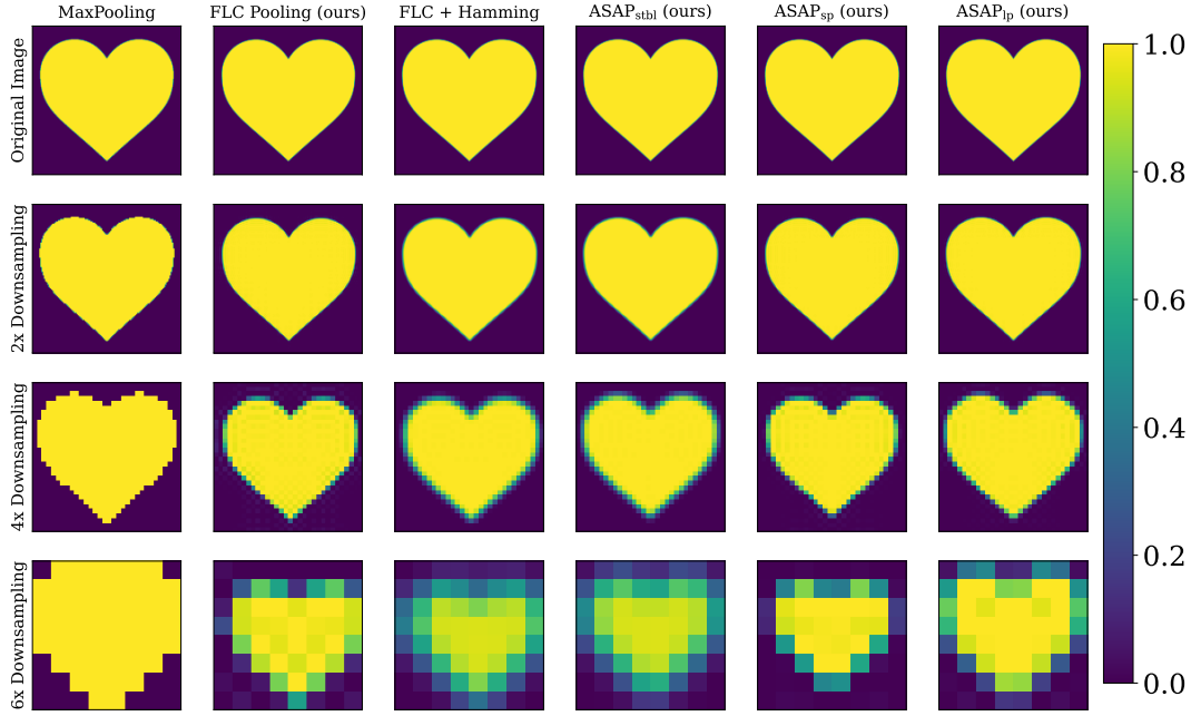
FIGURE 6.7: Qualitative Image Comparison of Different Downsampling Techniques. We qualitatively compare the influence of downsampling using different methods. The first column shows the commonly used MaxPooling. In the second column, we use FLC Pooling, and in the third column, we show FLC with an additional Hamming window applied. In the last three columns, we present our ASAP variants, which include the Hamming window and different stabilization techniques.
