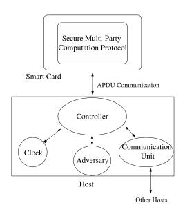
Fig. 3. Relations between architecture components.
