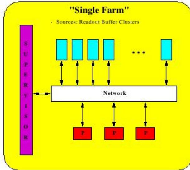
Fig. 1.11: Level2 Trigger Architecture C.
