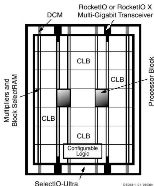
Fig. 4.3: A Generic Architecture Overview of modern FPGA (Xilinx Virtex2-Pro in this case).
