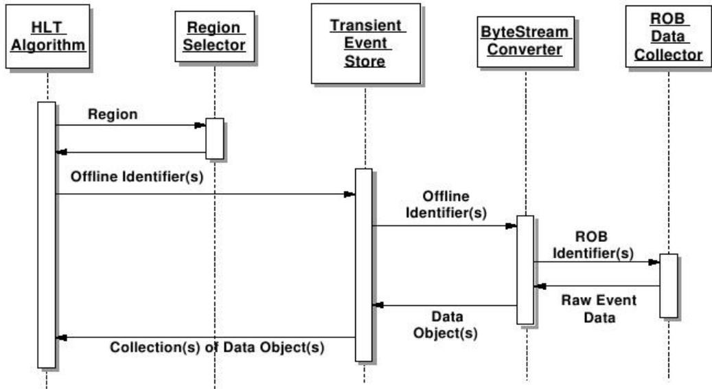
Fig. 3.3: A simplified schematic diagram of the sequence by which HLT algorithms request and receive event data.
