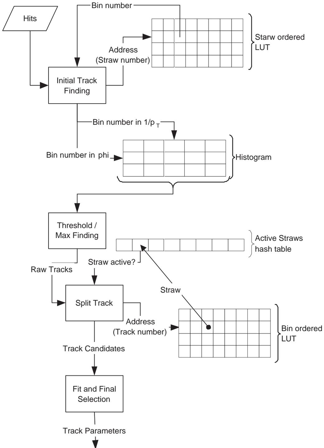
Fig. 6.3: TRT LUT-Hough algorithm
