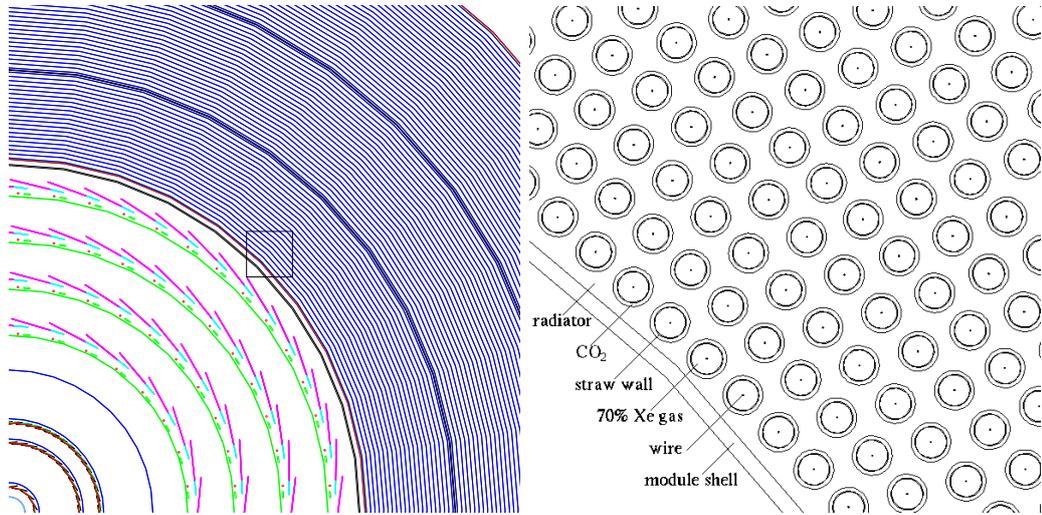
Fig. 1.5: TRT barrel geometry for simulation
