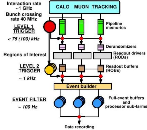
Fig. 1.7: Block diagram of the ATLAS Trigger/DAQ system.
