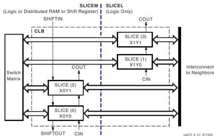
Fig. 4.1: Arrangement of Slices within the Xilinx Virtex-4 CLB.
