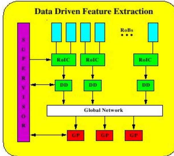
Fig. 1.9: Level2 Trigger Architecture A.
