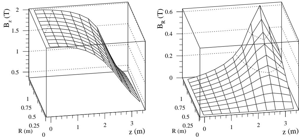
Fig. 1.6: Longitudinal and radial components of the magnetic field as a function of  $R$  and  $z$
