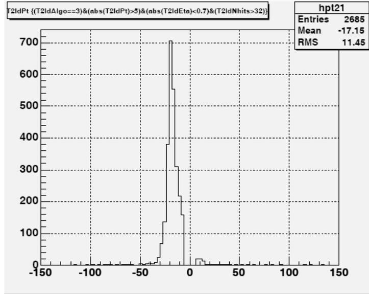
Fig. 6.14: Single 20 GeV electron events without pile-up. *Distribution of  $p_T$  for reconstructed tracks with  $|\eta| < 0.7$ . A number of generated events: 2758 (Efficiency: 97%)*
