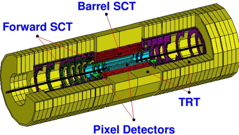
Fig. 1.2: The ATLAS Inner Detector
