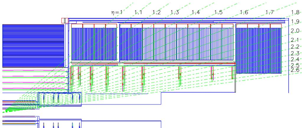
Fig. 6.9: View of one quarter of the ATLAS Inner Detector in the  $(R, z)$  plane.
