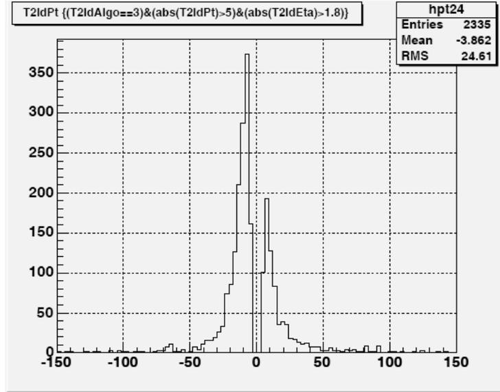
Fig. 6.13: Single 20 GeV electron events without pile-up. Distribution of  $p_T$  for reconstructed tracks with  $|\eta| > 1.8$ . LUT calculation done in case with an inhomogeneous magnetic field
