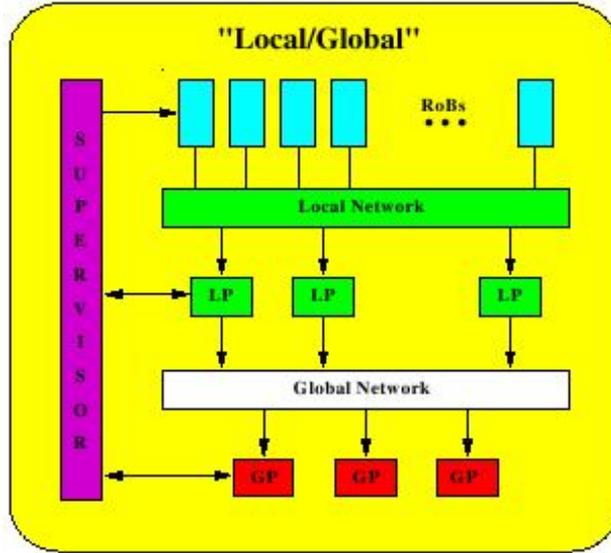
Fig. 1.10: Level2 Trigger Architecture B.
