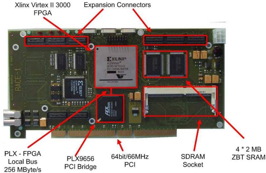
Fig. 4.4: Multi Purpose Reconfigurable Accelerator / Computing Engine
