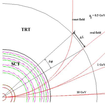
Fig. 6.11: Trajectories of the particles with various transverse momenta through the Inner Detector.  $R - \phi$  view.
