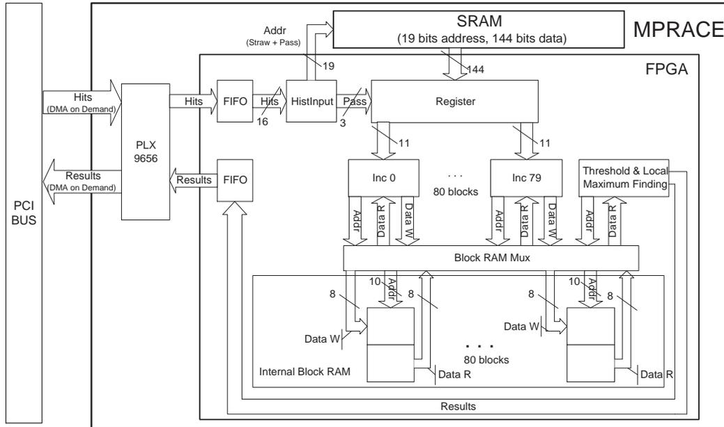
Fig. 6.4: FPGA initial track finding
