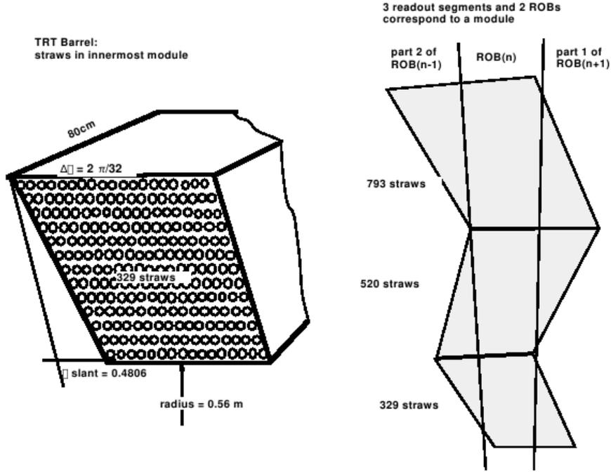
Fig. 1.4: TRT barrel modules (mechanical layout)
