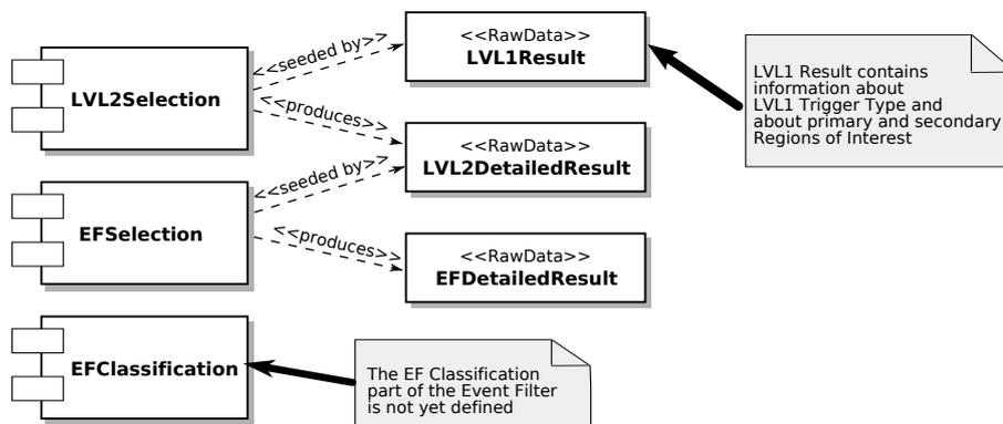
Fig. 3.1: A component diagram of the High Level Trigger selection chain
