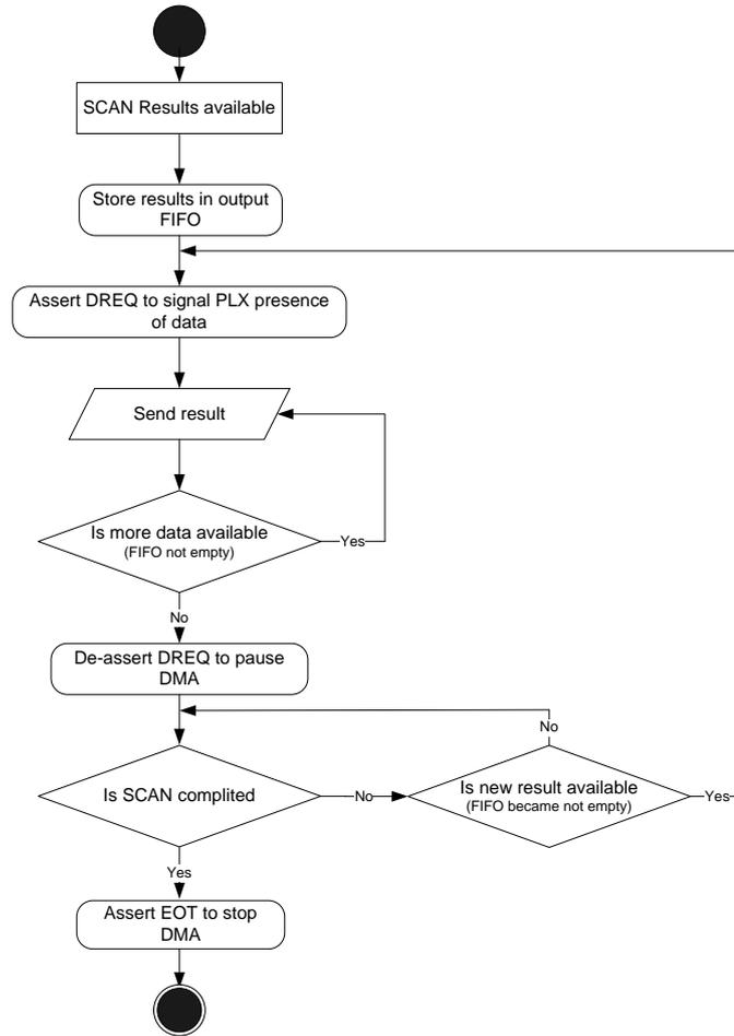
Fig. 6.7: Flow diagram of the DMA-on-demand data transfer
