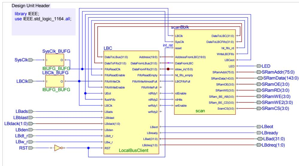
Fig. 6.5: TRT LUT-Hough initial track finding block diagram
