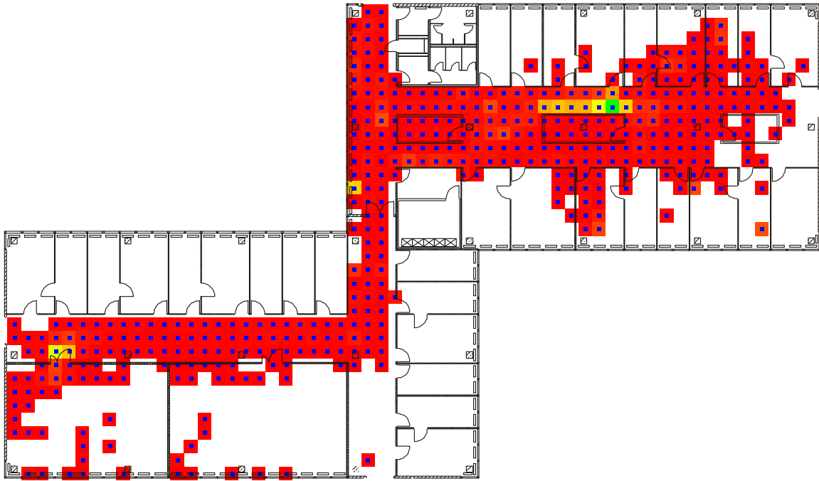
Figure 6.12: Overview of areas within our test bed that are especially susceptible to large errors.
