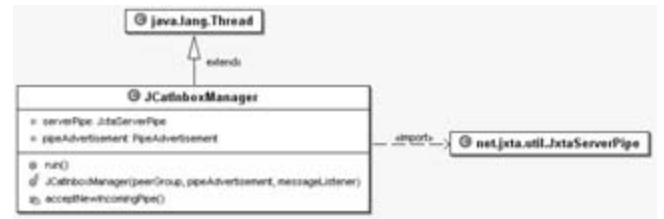
Figure 9: UML diagram of the Juxta-CAT Inbox manager.
